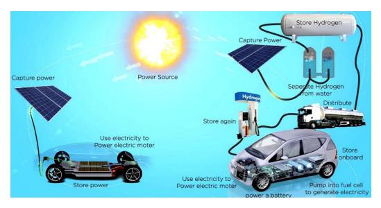
*Figure 1:* Left, power mechanism of battery electric vehicle. Right, power mechanism of hydrogen fuel-cell electric vehicle (Image: <u>www.aveq.ca</u>).
