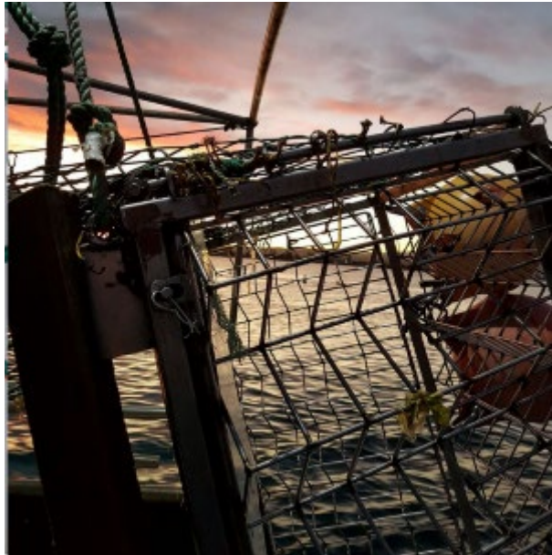
Figure 20: Rigid cod-end with rectangular openings. Image credit: Karl Warr/Better Fishing Co.
